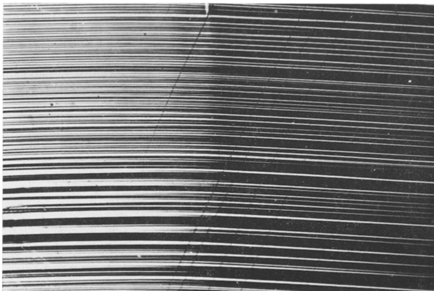
Figure 13 Bending associated with the tapered martensite plates. The black areas correspond to the untransformed \beta -Cu-Zn-Al phase whilst the white lamellae are the martensite plates.
